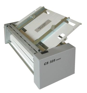
The machine has one feeding table and one holder for gripping of cutting tools. Sheets are inserted manually to the machine, sheet by sheet.
